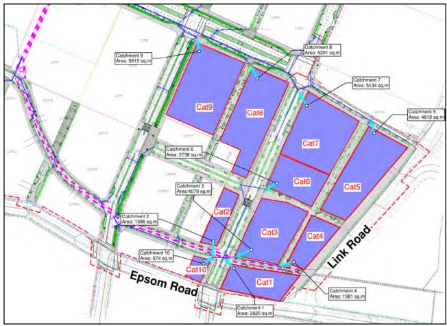
Figure 7 – Proposed Sub-Catchment Plan and Points of Discharge to the Council Stormwater System
