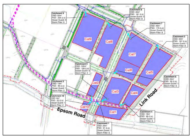
Figure 11 – Proposed Stormwater Concept Plan
